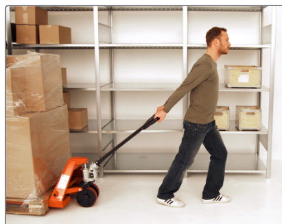
When the pallet truck starts to move, turn around and pull it along after you.
