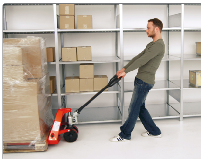
To start the pallet truck, stand with one foot in front of the other as if you were taking a step - then lean back and keep your arms straight.
