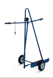
Board trolleys have two or four wheels and are designed specifically to transport long and large items such as furniture cases, boards, sheet panels, mattresses and mirrors. Board trolleys can be used in the shop area, in the stockroom and when receiving and delivering goods. They are specifically suited for transporting boards and similar in an upright position.
