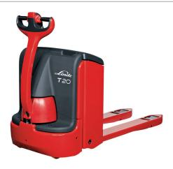
A powered pallet truck is battery powered and the forks can be raised approx. 150mm from the floor. The pallet truck comes with forks of various lengths and takes up slightly more space than a hand pallet truck. Powered pallet trucks can be used to transport products over longer distances indoors and outdoors, as well as to transport heavy pallets and to transport pallets on gently sloping surfaces.
